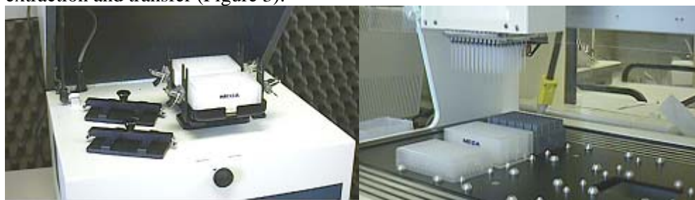
Figure 3. (Left) Tissue is macerated in a genogrinder, which processes two plates at one time. (Right) Extracted DNA is transferred from sample plates to storage plates using robotics.
