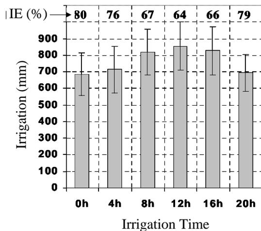
**Figure 4.** Effect of the time of sprinkler irrigation on the irrigation depth required to obtain maximum maize yield in the conditions of Zaragoza, Spain. Irrigation efficiency estimates are supplied for each case at the top of the figure.
