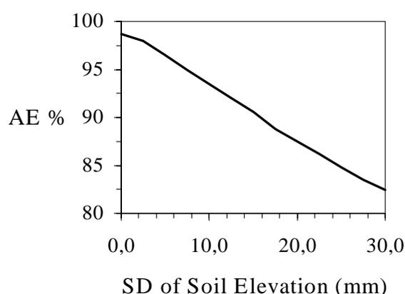
**Figure 3. Simulated effect of the quality of land leveling (characterized by the standard deviation of soil surface elevation) on application efficiency in a particular case of level-basin irrigation.**
